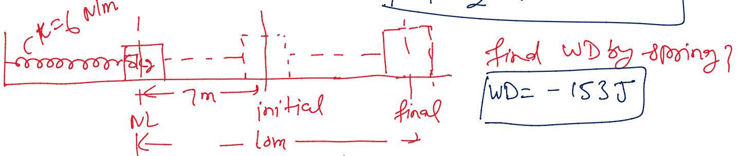
Area under force-displacement curve :-
