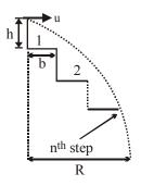
Let t be the time taken by the ball for these horizontal and vertical displacement. Then velocity along horizontal direction remains constant = u; initial vertical velocity is zero
