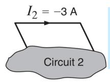
A NEGATIVE VALUE FOR THE CURRENT INDICATES FLOW IN THE OPPOSITE DIRECTION THAN THE REFERENCE DIRECTION
