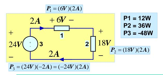
Tellegen's theorem: the sum of the powers absorbed by all elements in an electrical network is zero. Another statement of this theorem is that the power supplied in a network is exactly equal to the power absorbed.
