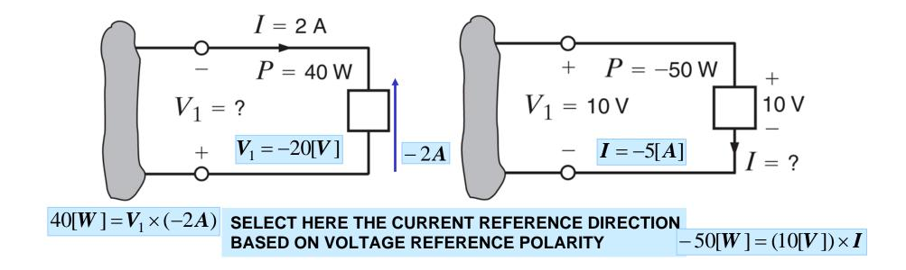
WHICH TERMINAL HAS HIGHER VOLTAGE AND WHICH IS THE CURRENT FLOW DIRECTION
