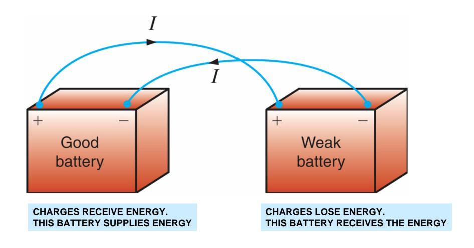
WHAT WOULD HAPPEN IF THE CONNECTIONS ARE REVERSED IN ONE OF THE BATTERIES?
