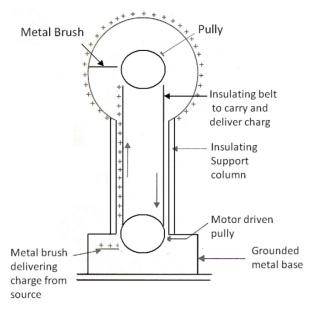
As shown in the figure a spherical shell of a few meter radius, is kept on an insulated support, at a height of a few meters from the ground.
