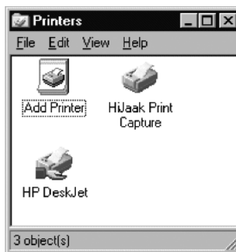
Figure 2: The Add Printer Wizard lets you configure local print devices and remote access to network printer servers.
