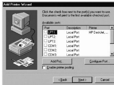
Figure 3: In the Add Printer Wizard window, select a printer port for a local printer or click on the Add Port button for a network-attached printer.
