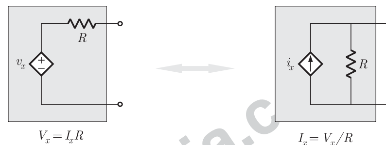
Fig. 5.4.4 Source Transformation of Dependent Sources
