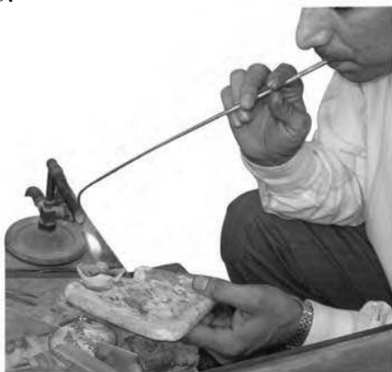
Fig. 6.11 : Goldsmith blowing through a metallic pipe
