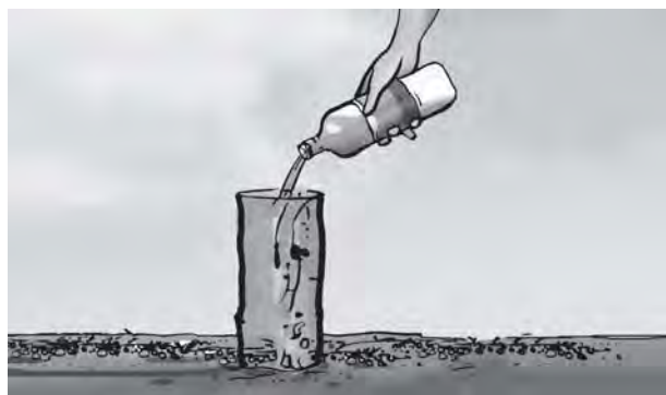
Fig. 9.5 Measuring rate of percolation
