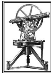
A Theodolite (Surveying instrument, which is based on the Principles of trigonometry, is used for measuring angles with a rotating telescope)
