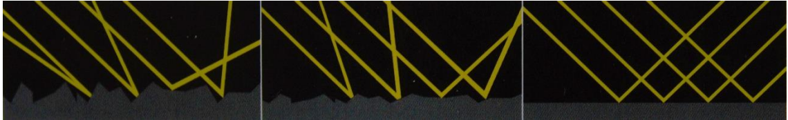
Figure 1. Microfacet models expressing the lights behaviour in diffuse, glossy and specular reflection. (Birn 2014, 315)
