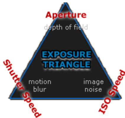
Picture 9. The relation of aperture, shutter speed and ISO value to each other and to the exposure. (Cambridge in Colour 2016b).
