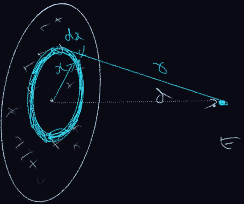
$$dV = \frac{k dq}{x} = \frac{k (\sigma 2\pi x dx)}{\sqrt{x^2 + d^2}}$$
