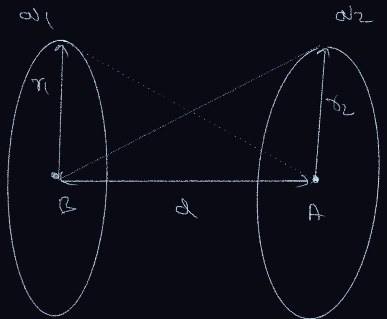
$$\omega_A = \kappa \left( \frac{\omega_2}{\sigma_2} + \frac{\omega_1}{\sqrt{d^2 + \sigma_1^2}} \right)$$
