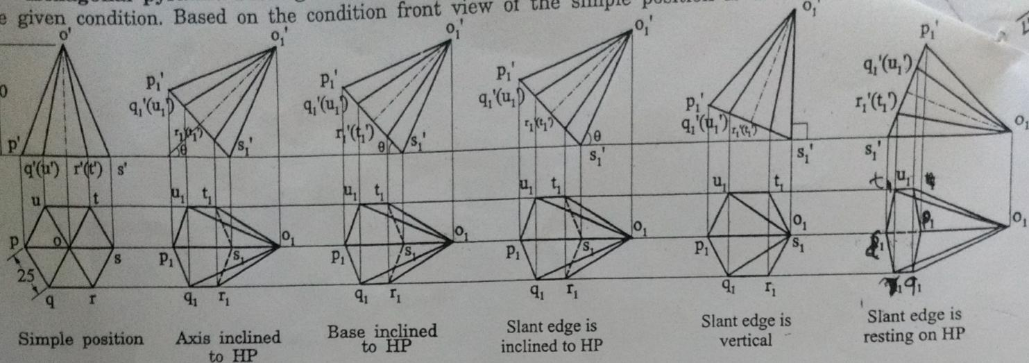
**Hexagonal pyramid resting on one of its corner on VP.** Simple position is common for all the given condition. Based on the condition top view of the simple position is tilted
