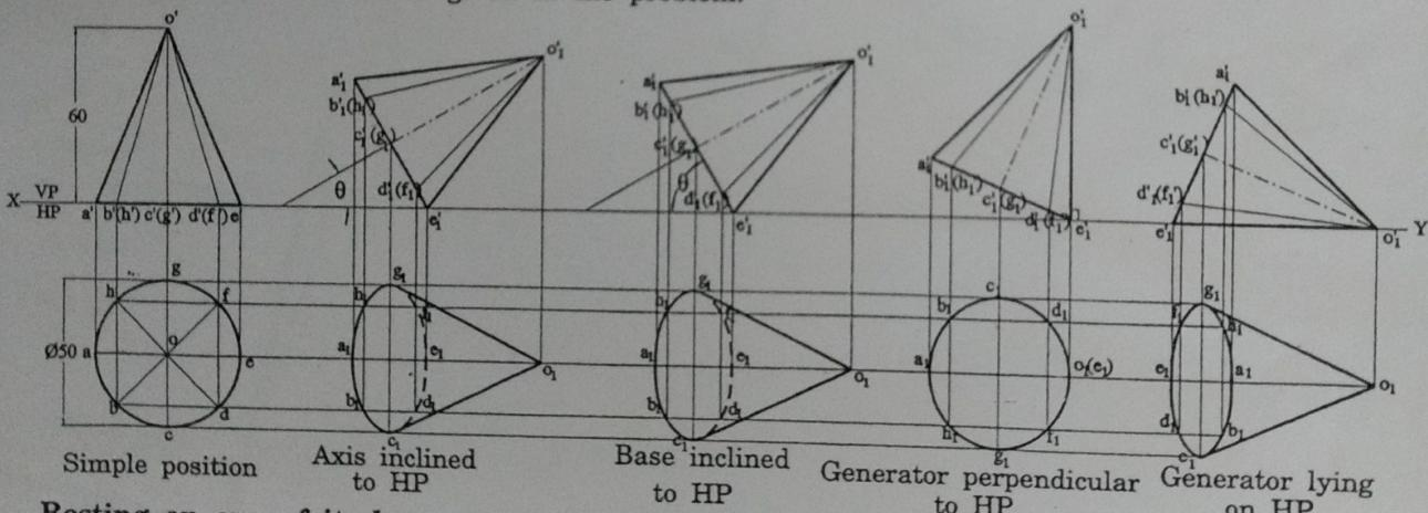
**Resting on one of its base point VP.** Draw the simple position as given below. Tilt the top view of the cone for the conditions given in the problem.
