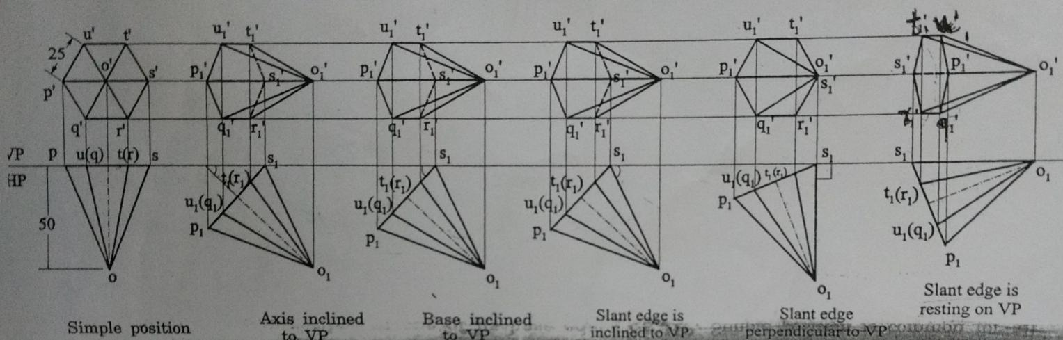
**Cone resting on one of its base point on HP.** Draw the simple position as given below. Tilt the front view of the cone for the conditions given in the problem.
