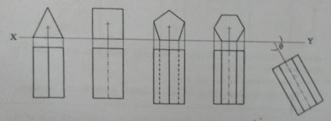
Resting on one of the rectangular face on VP and axis or base is inclined
