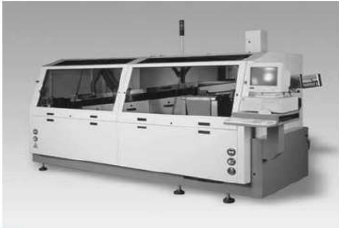
FIGURE 17.32 Wave-soldering machine. (Picture courtesy of Sincotron, Vitronics Soltec DeltaMax)
