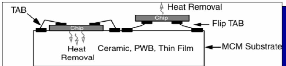
**(c) tape automated bonding (TAB)**
