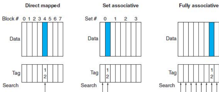
FIGURE 5.14 The location of a memory block whose address is 12 in a cache with eight blocks varies for direct-mapped, set-associative, and fully associative placement. In direct-mapped placement, there is only one cache block where memory block 12 can be found, and that block is given by (12 \bmod 8) = 4 . In a two-way set-associative cache, there would be four sets, and memory block 12 must be in set (12 \bmod 4) = 0 ; the memory block could be in either element of the set. In a fully associative placement, the memory block for block address 12 can appear in any of the eight cache blocks.
