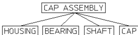
Figure 246. Cap Bearing Parts Structure
