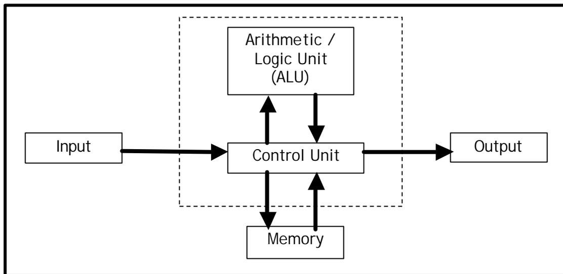
Figure 1-1 Functional Components of a Computer
