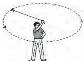
Fig. 8.10: A stone describing a circular path with a velocity of constant magnitude.
