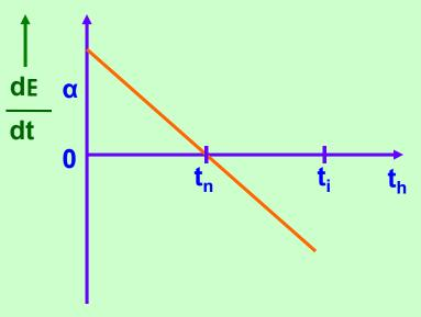
The graph between Seebeck power and temperature is a straight line and is called 'thermoelectric power line'.
