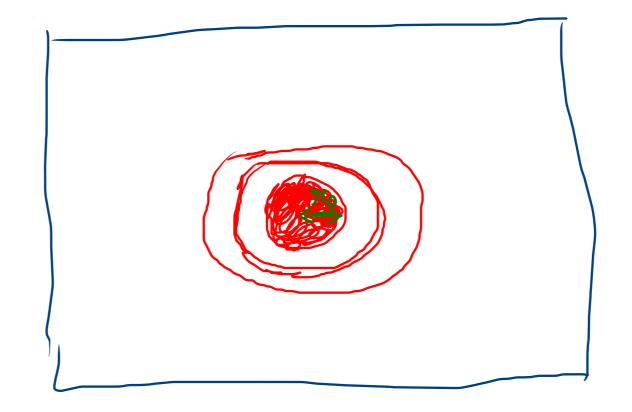
Due to diffraction instead of a point, the parllel rays will focus at a spot of finite area
