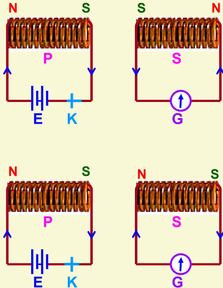
When the primary circuit is closed current grows from zero to maximum value.
