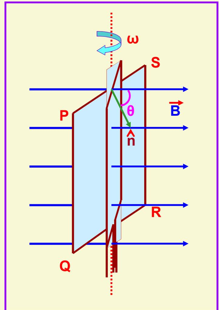
The emf changes continuously in magnitude and periodically in direction w.r.t. time giving rise to alternating emf.
