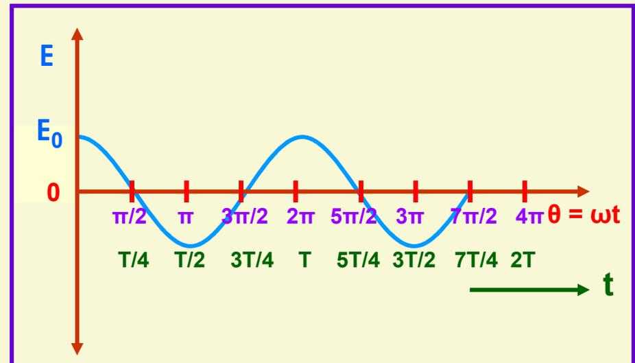
This method of inducing emf is the basic principle of generators.
