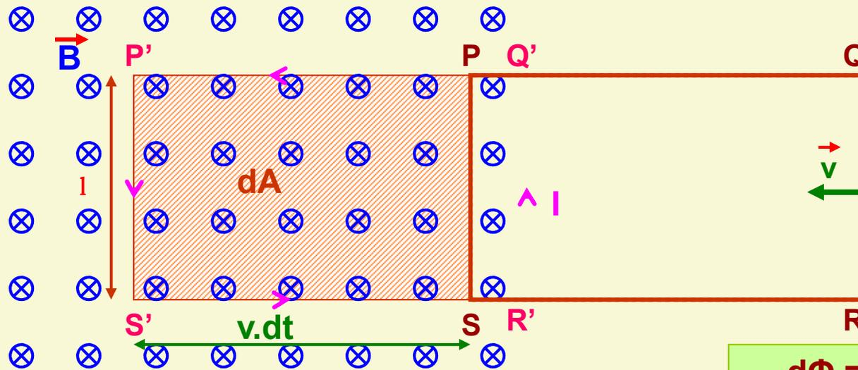
The loop PQRS is slid into uniform and perpendicular magnetic field. The change (increase) in area of the coil under the influence of the field is  $dA$  in time  $dt$ . This causes an increase in magnetic flux  $d\Phi$ .
