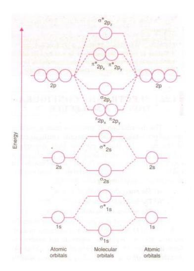
Molecular orbital energy level diagram for  $O_2$ ,  $F_2$ ,  $Ne_2\,$  etc.
