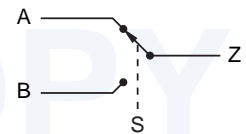
Figure 1-7 Switch model for multiplexer function.
