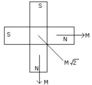
Resultant moment of inertia of both the magnets about the axis of rotation will be 2I, where 'I' is the moment of inertia of each magnet.
