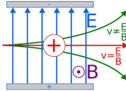
This particle is deflected downwards with a force  $FB = qvB$ . When these two forces are equal the particle is not deflected in any direction.  $qvB = qE$ ,  $v = E/B$ . Hence particles with velocity 'v' only will be coming out through the straight path. Velocity selector is used in accelerator mass spectroscopy to select particles of a particular velocity.
