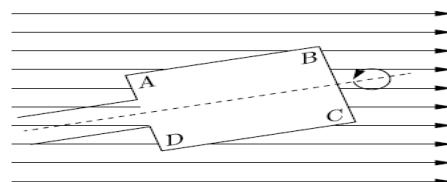
7. A rectangular coil  $ABCD$  is rotated anticlockwise with a uniform angular velocity about the axis shown in the figure. Initially, the axis of rotation of the coil as well as the magnetic field  $B$  were horizontal. The induced e.m.f. in the coil would be maximum when plane of the coil
