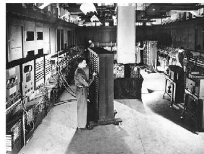
6. ENIAC was therefore about 1,000 times faster than the previous generation of relay computers. ENIAC used **18,000 vacuum tubes** about 1,800 square feet of floor space, and consumed about 180,000 watts of electrical power.
