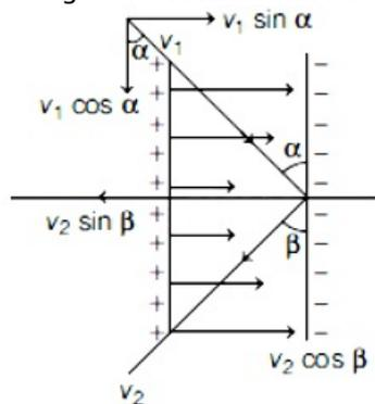
Let,  $v_1$  and  $v_2$  be the incoming and outgoing velocities of electron into the capacitor and out of the capacitor, respectively. Since, electric field is along X-axis, hence electric force on electron along Y-axis,  $(F_y) = 0$
