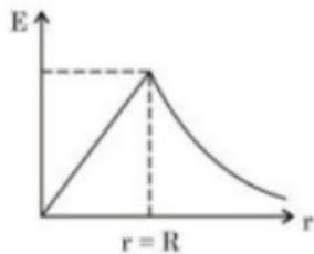
Electric field due to uniformly charged insulating solid sphere
