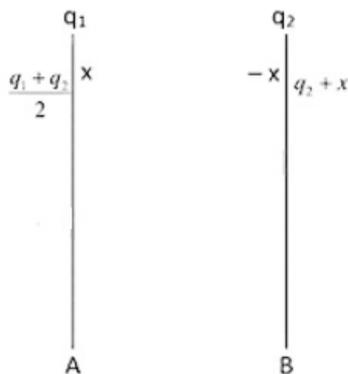
$$\text{Charge on the left surface of plate A} = \frac{\text{Total charge}}{2} = \frac{q_1 + q_2}{2}$$
