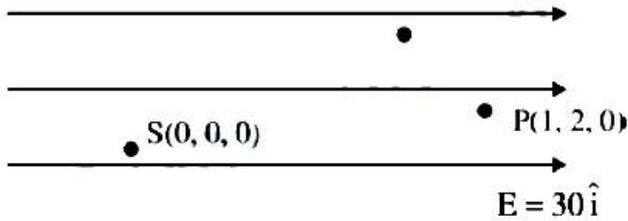
$$\begin{aligned}\omega_E &= q\vec{E} \cdot \vec{S} \\ &= 2 \times 10^{-2} [30 \hat{i} \cdot (-\hat{i})] \\ &= 2 \times 10^{-2} (-30) \\ &= -60 \times 10^{-2} \\ &= -\frac{60}{100} = -0.6\text{J} \\ &= -600\text{mJ}\end{aligned}$$
