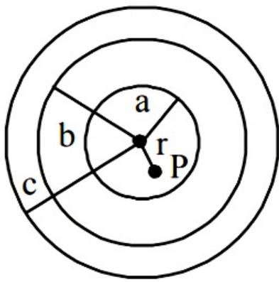
Potential at point P,  $V = \frac{kQ_a}{a} + \frac{kQ_b}{b} + \frac{kQ_c}{c}$
