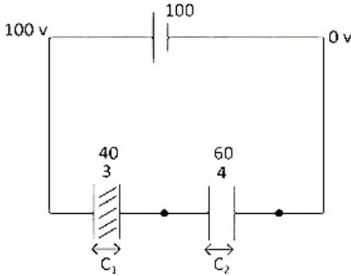
$$\frac{C_1}{C_2} = \frac{3 \times t_2}{t_1 \times 4} = \frac{3}{2}$$
