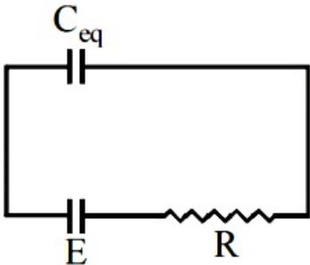
During charging charge on the capacitor increases with time. Charge on the capacitor  $C_1$  as a function of time,
