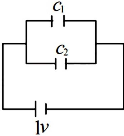
$$\frac{U_1}{U_2} = \frac{\left(\frac{1}{2}C_1V^2\right)}{\left(\frac{1}{2}C_2V^2\right)} = \frac{1}{4} \Rightarrow \frac{C_1}{C_2} = \frac{1}{4}$$
