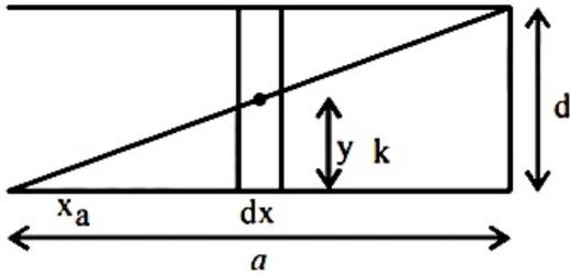
From figure,  $\frac{y}{x} = \frac{d}{a} \Rightarrow y = \frac{d}{a}x$
