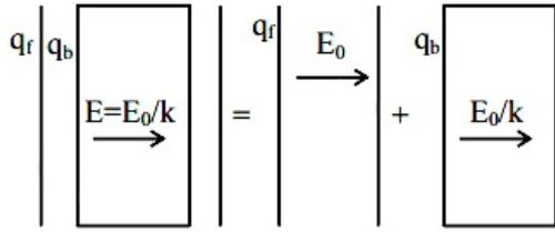
When a dielectric is inserted in a capacitor
