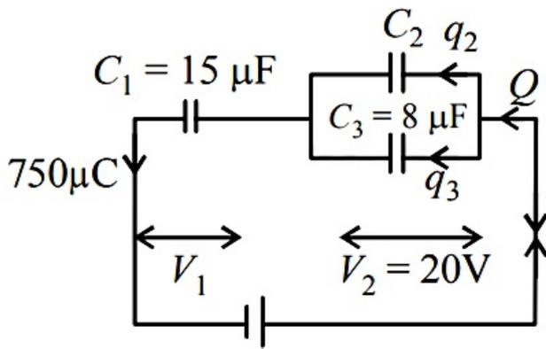
Capacitors  $C_2$  and  $C_3$  are in parallel hence,
