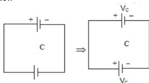
$$V_c = \frac{C_1 V_1 + C_2 V_2}{C_1 + C_2}$$
