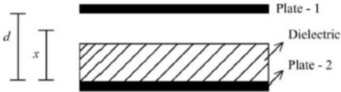
Let  $C_1$  and  $C_2$  be the capacitance of the system for  $x = \frac{1}{3}d$  and  $x = \frac{2d}{3}$ , respectively. If  $C_1 = 2\mu\text{F}$  the value of  $C_2$  is \_\_\_\_\_  $\mu\text{F}$
