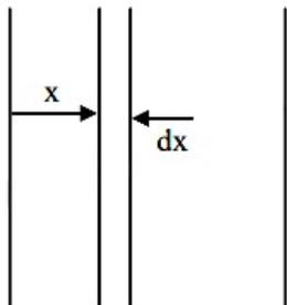
Taking an element of width  $dx$  at a distance  $x$  ( $x < d/2$ ) from left plate
