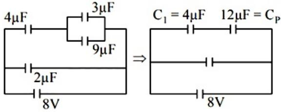
$$\text{Charge on } C_1 \text{ is } q_1 = \left[ \left( \frac{12}{4 + 12} \right) \times 8 \right] \times 4 = 24 \mu\text{C}$$
