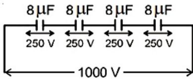
$$\frac{1}{C_{\text{eq}}} = \frac{1}{8} + \frac{1}{8} + \frac{1}{8} + \frac{1}{8} \therefore C_{\text{eq}} = 2\mu\text{F}$$
