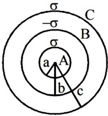
$$V_B = \frac{K q_A}{r_b} + \frac{K q_B}{r_b} + \frac{K q_C}{r_c}$$
