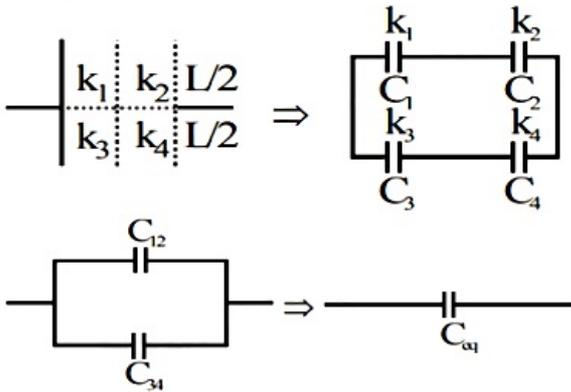
$$C_{12} = \frac{C_1 C_2}{C_1 + C_2} = \frac{k_1 \epsilon_0 \frac{L}{2} \times L}{d/2} \cdot \frac{k_2 \left[ \epsilon_0 \frac{L}{2} \times L \right]}{d/2} \frac{1}{(k_1 + k_2) \left[ \frac{\epsilon_0 \frac{L}{2} \times L}{d/2} \right]}$$
