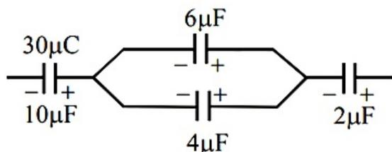
As given in the figure,  $6 \mu\text{F}$  and  $4 \mu\text{F}$  are in parallel. Now using charge conservation
