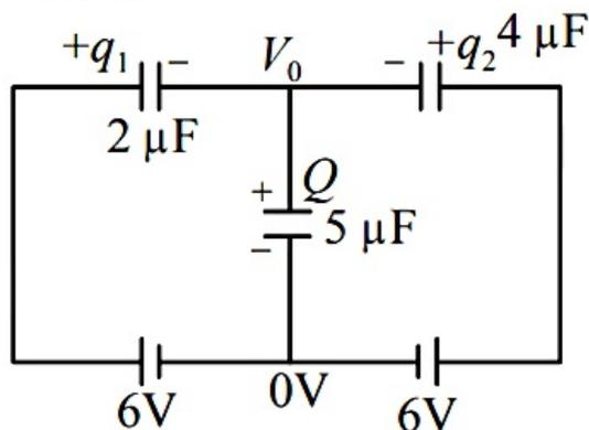
Let  $q_1$  and  $q_2$  be the charge on the capacitors of  $2\mu\text{F}$  and  $4\mu\text{F}$ . Then charge on capacitor of  $5\mu\text{F}$
