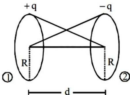
Potential at the center of ring of charge +q = potential due to it self + potential due to other ring of charge -q.
