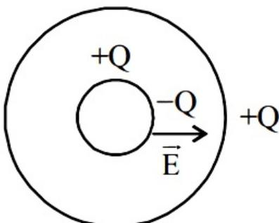
Electric field between spherical surface  $\vec{E} = \frac{KQ}{r^2}$  So  $\int \vec{E} \cdot d\vec{r} = V$  given
