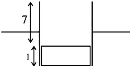
$$\begin{aligned}C_{\text{eff}} &= \left[ \frac{\epsilon_0(7 \times 4)}{4/10} + \frac{5\epsilon_0(1 \times 4)}{4/10} \right] \times 10^{-2} \\ C_{\text{eff}} &= 1.2\epsilon_0 \\ \text{Energy} &= \frac{1}{2}C_{\text{eff}}V^2 \\ &= \frac{1}{2}(1.2)\epsilon_0(20)(20) = 240\epsilon_0\end{aligned}$$
