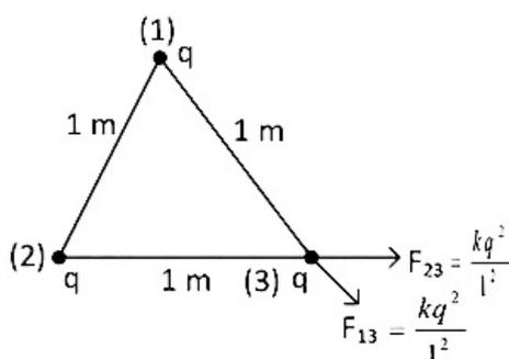
$$F_{\text{net}} \text{ on charge 3, } F_1 = \frac{\sqrt{3}kq^2}{1^2}$$
