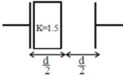
$$\begin{aligned} C_{\text{new}} &= \frac{E_0 A}{\frac{\left(\frac{d}{2}\right)}{1.5} + \frac{\left(\frac{d}{2}\right)}{1}} \\ &= \frac{E_0 A}{\left(\frac{d}{3} + \frac{d}{2}\right)} = \frac{6E_0 A}{5d} \\ &= \frac{6}{5} \times 5\mu F = 6\mu F \end{aligned}$$
