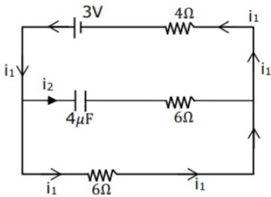
In steady state, no current will pass through capacitor hence capacitor will act as open circuit.
