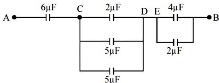
The equivalent capacitance between C&D capacitors of  $2\mu\text{F}$ ,  $5\mu\text{F}$  and  $5\mu\text{F}$  are in parallel.
