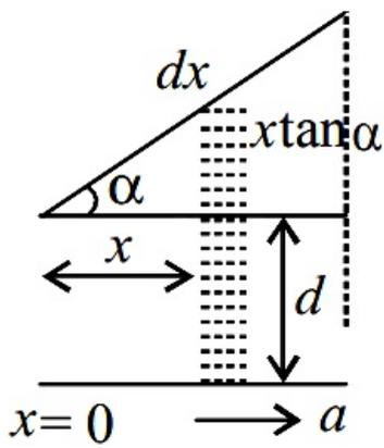
Consider an infinitesimal strip of capacitor of thickness  $dx$  at a distance  $x$  as shown.
