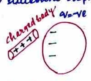
Step-3:- uncharged body is disconnected from earth.
