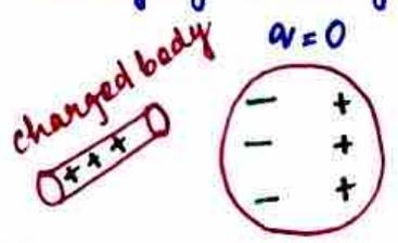
Step-1:- charged body is brought near an uncharged body.
