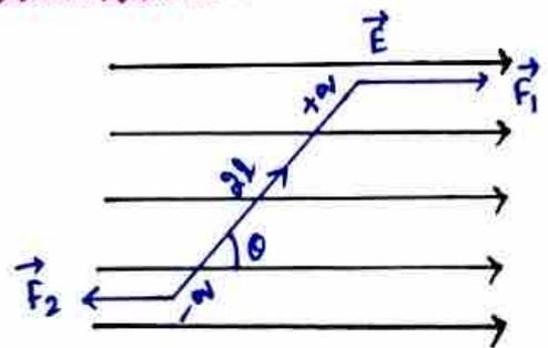
$\theta$  is the angle between dipole moment and intensity.
