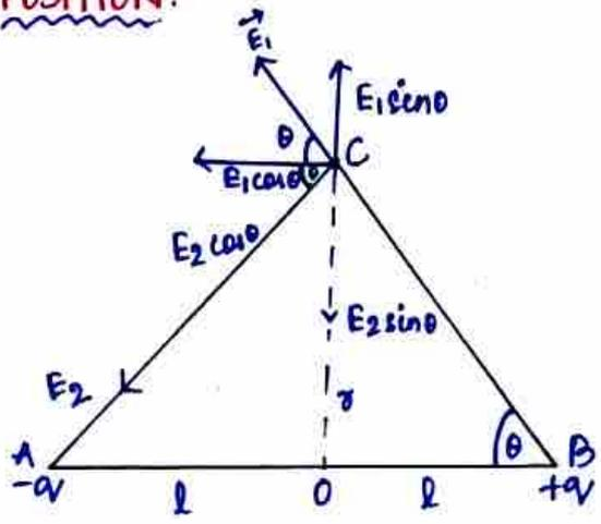
C is any point on the equatorial line at a distance r from the centre of the dipole.
