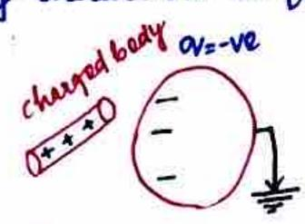
Step-2:- uncharged body is connected to earth.
