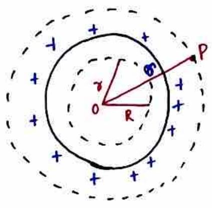
This expression is same as the expression used in intensity due to point charge. So charges resides on the surface of the spherical shell behave as if they are concentrated at the centre.
