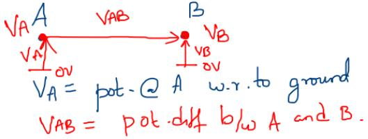
$$V_A, V_B = \text{pot. / when w.r.t. to ground}$$
