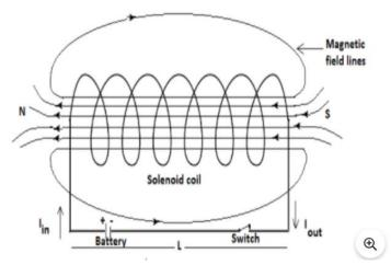
The field lines inside the solenoid are in the form of straight parallel lines showing uniform magnetic field.
