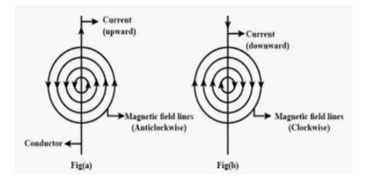
• If we hold a straight current conductor in our right hand such that the thumb represents the direction of current then the fingers encircling represent the direction of magnetic field lines.
