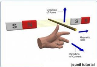
If we stretch our thumb, index finger and the central finger of our left hand such that they are mutually perpendicular to each other, if the index finger represents the direction of magnetic field and the central finger represents the direction of current then the thumb represents the direction of Force experienced by the conductor.
