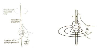
Current – upwards, Magnetic field lines – anticlockwise direction Current – downwards, Magnetic field lines – clockwise direction
