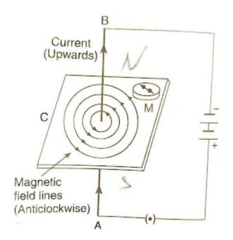
The shape of field lines is in form of concentric circles (around a common) center
