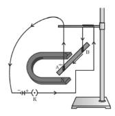
In the above figure, a current-carrying rod, AB, experiences a force perpendicular to its length and the magnetic field.
