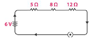
Q4. Redraw the circuit of Question 1, putting in an ammeter to measure the current through the resistors and a voltmeter to measure the potential difference across the 12  $\Omega$  resistor. What would be the readings in the ammeter and the voltmeter
