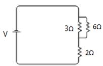
From the circuit above, it is understood that 3  $\Omega$  and 6  $\Omega$  are connected in parallel. Hence, their equivalent resistance is given by
