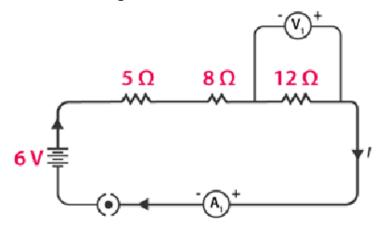
Using Ohm's Law, we can obtain the reading of the ammeter and the voltmeter.
