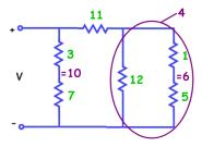
We see on the right that the total resistance 6 and the resistor 12 are now in parallel. We can solve for these parallel resistors to get the equivalent resistance of 4.
