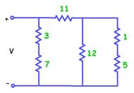
First we will total the two series resistors on the right (1 + 5 = 6) and on the left (3 + 7 = 10). Now we have reduced the circuit.
