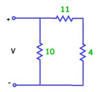
From this circuit we solve for the series resistors 4 and 11 to get 4 + 11 = 15. Now we have two parallel resistors, 15 and 10.
