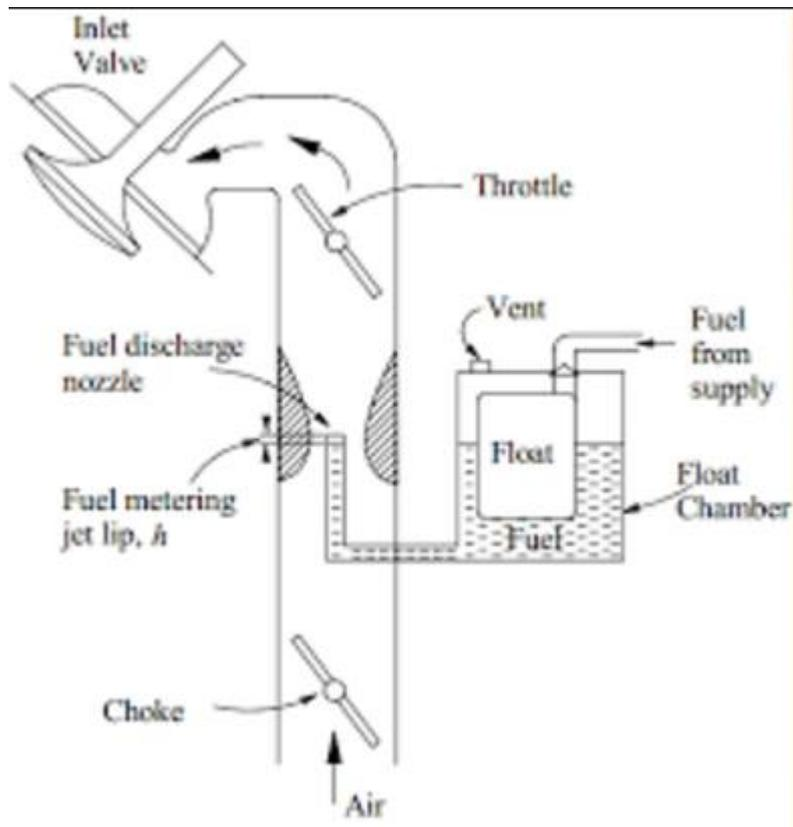
Throttle valve is used to control how much mass enters the cylinder. It is controlled by Governors. Function of governor is to increase / decrease the amount of mixture entering the cylinder.
