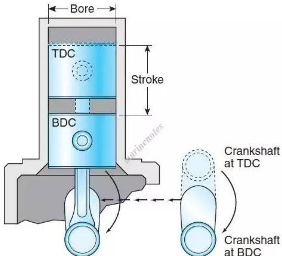
Stroke to bore ratio (L/d ratio):
