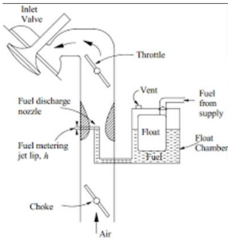
When choke valve is closed, it means it is obstructing the flow (see image in #12).
