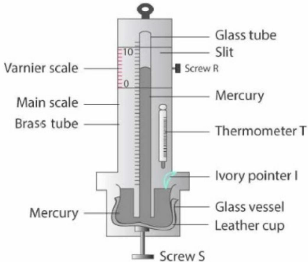
The leather cup is raised up or lowered down first to measure the atmospheric pressure, it is done using a screw S so that the ivory pointer I just touches the level of mercury in the glass vessel. The point of the mercury level in the barometer tube is observed using the main scale and the vernier scale. The addition of the vernier scale reading to the main scale reading yields barometric height.
