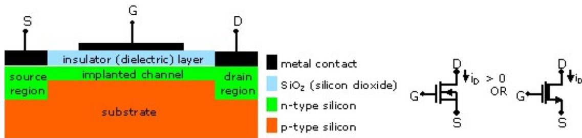
**n-channel depletion MOSFET (depletion NMOS)**
