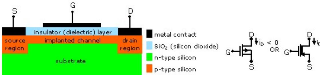
**p-channel depletion MOSFET (depletion PMOS)**
