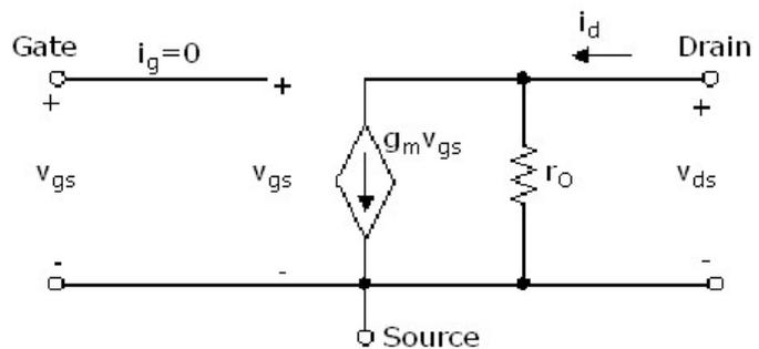
$$g_m = \frac{\partial i_d}{\partial v_{gs}} = -\frac{2I_{DSS}}{V_P} \left( 1 - \frac{V_{GS}}{V_P} \right) (1 + \lambda v_{DS})$$
