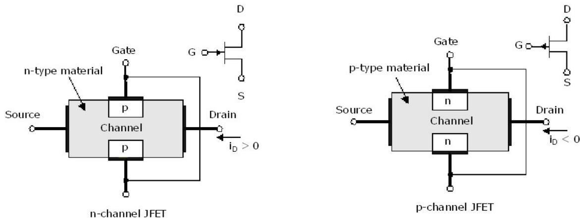
Like the BJT, the JFET is a three terminal device. Although there are physically two gate diffusions, they are tied together and act as a single **gate** terminal. The other two contacts, the **drain** and **source**, are placed at either end of the channel region. The JFET is a symmetric device (the source and drain may be interchanged), however it is useful in circuit design to designate the terminals as shown in the circuit symbols above.
