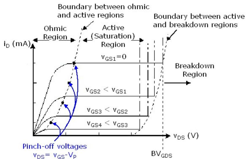
Below pinch-off, the channel essentially behaves like a constant resistance as we discussed earlier. This linear region of operation is called **ohmic** (or sometimes triode), and is where the JFET may be used as a resistor whose value is determined by the value of  $v_{GS}$ . The
