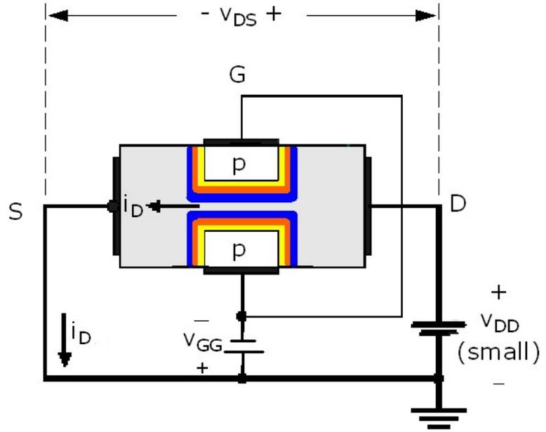
If we now apply the  $v_{DS}$  variation effect, we can see that pinch-off will occur for lower values of  $v_{DS}$  since we have less of a channel to start with (resulting in lower values of  $i_D$  at pinch-off). By combining the effect of  $v_{DS}$  and  $v_{GS}$  variations, a family of characteristic curves similar to the figure at the right (based on Figure 6.16a of your text) will be generated for the n-channel JFET.
