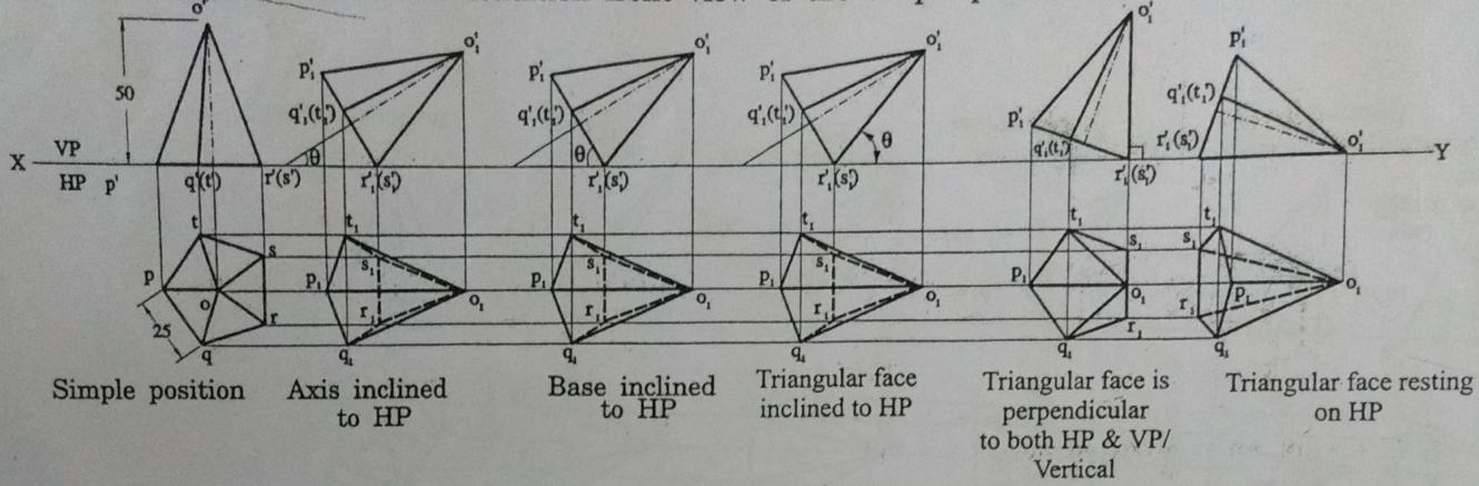
**Pentagonal pyramid resting on one of its base edge on VP.** Here simple position is common for all the given condition. Based on the condition top view of the simple position is tilted.
