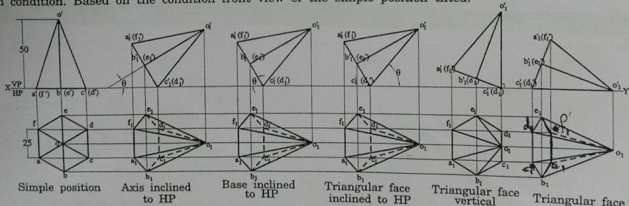
**Hexagonal pyramid resting on one of its base edge on VP.** Simple position is common for all the given condition. Based on the condition top view of the simple position tilted
