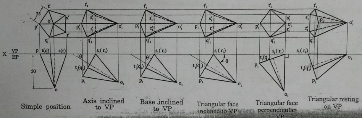
**Hexagonal pyramid resting on one of its base edges on HP.** Simple position is common for all the given condition. Based on the condition front view of the simple position tilted.
