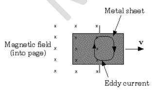
1. Eddy current is the outcome of Lorentz magnetic force, In above example V and B is perpendicular to each other hence charge is acted upon by magnetic force which make it move in circular orbit
