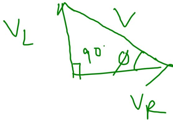
$$\begin{aligned} \tan \phi &= \frac{V_L}{V_R} \\ &= \frac{IX_2}{IR} = \frac{X_2}{R} \end{aligned}$$
