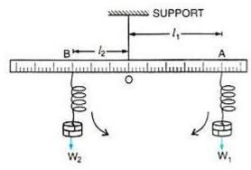
Let the weight suspended on the right side of thread from the spring balance at A be  $W_1$  at distance  $OA = l_1$ , while the weight suspended on the left side of thread from the spring balance at B be  $W_2$  at distance  $OB = l_2$ .
