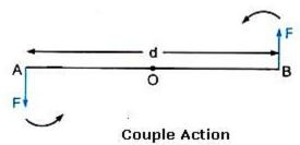
At A and B, two equal and opposite forces each of magnitude F are applied. The two forces rotate the bar in anticlockwise direction. The perpendicular distance between two forces is AB
