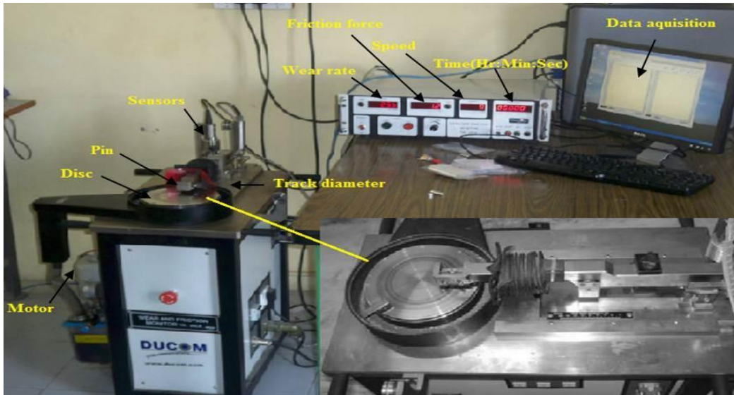
Figure 5. ‘Pin-on-Disc’ wear testing machine
