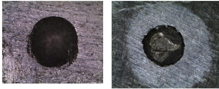
FIGURE 6. Front end appearance of target after ballistic testing
