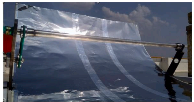
Fig. 4. Fabricated parabolic trough collector with rotary receiver tube.
