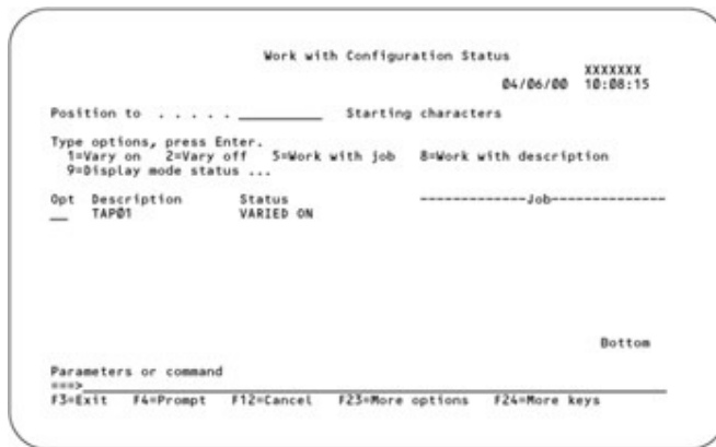
Figure 6.15: Work with Configuration Status Screen (Tape Devices)
