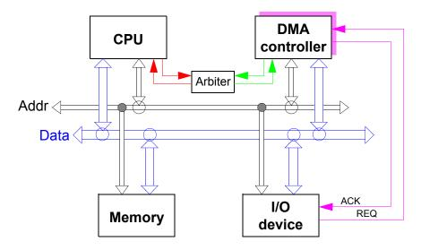
simplified logical structure of a system with DMA
