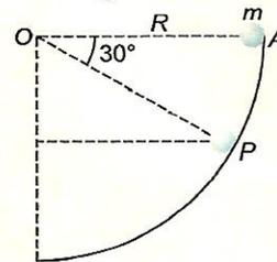
It is released from rest at A, the normal contact force exerted by surface on particle when it reaches P is
