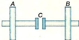
moment of inertia of A is half of that of B. When the clutch is in disconnected position, the disk A is brought up to an angular velocity  $\omega_0$  with the help of an external torque. Then external torque is removed from A and it is coupled to B with the help of clutch. Neglect bearing friction in the shaft but due to coupling 150 J of heat is developed in the clutch. The initial kinetic energy (just before the connections are made) of the disk A was (Assume clutch and shaft are light).
