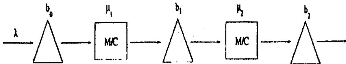
**Fig. Two-machine-one buffer-system.**
