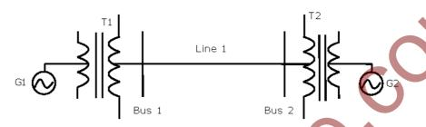
Choose 25 kV as the base voltage at the generator G1, and 200 MVA as the MVA base. The impedance diagram is
