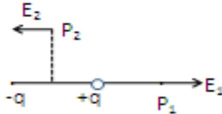
The direction of electric field  $E_1$  at axial point  $P_1$  and electric field  $E_2$  at equatorial point  $P_2$  are shown in fig. Obviously, angle between  $E_1$  and  $E_2$  is  $180^\circ$
