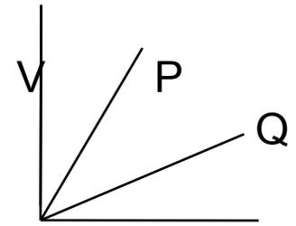
18) V-I graph for a metallic wire at two different temperatures  $T_1$  and  $T_2$  is shown in the figure. Which of these two temperatures is higher and why?
