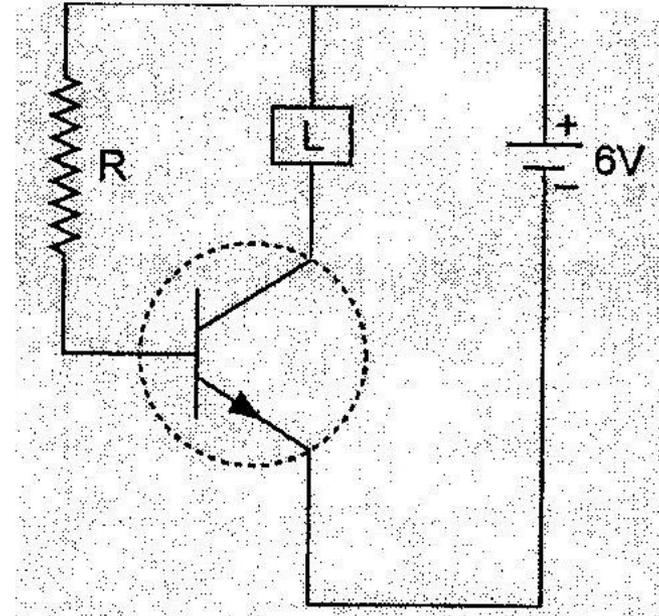
In (i) circuit, the emitter base junction is not biased, so no current flows across  $L$ ; hence lamp  $L$  does not light. In (ii) circuit, the emitter base junction is forward biased, so emitter and hence collector current flows and lamp  $L$  lights up.
