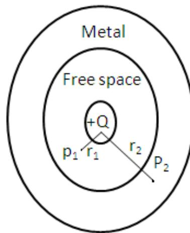
Now consider a spherical surface of radius  $r_2$  such that  $QP_2 = r_2$  charge induced on inner surface of metallic sphere =  $-Q$
