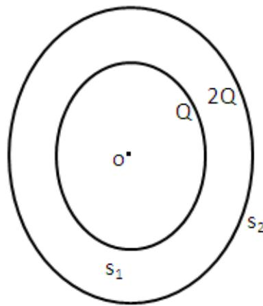
i) Surface  $S_1$  encloses charge  $Q$  only, therefore, electric flux through  $S_1$  is  $\Phi_1 = Q / \epsilon_0$
